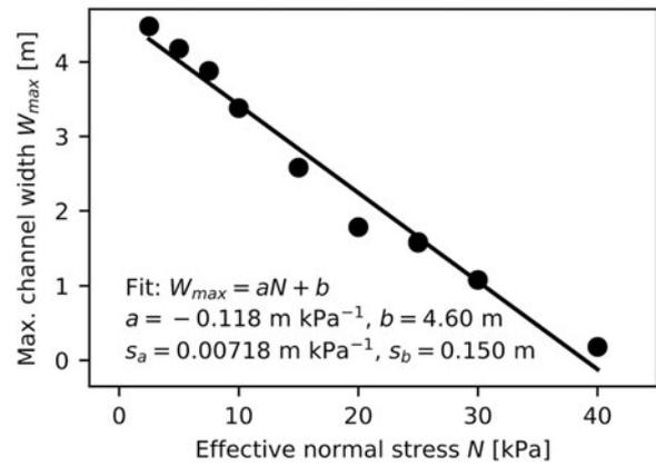
**Fig. 7.** Observed maximum channel width,  $W_{max}$ , under a constant imposed value for effective normal stress,  $N$ . Data points are fitted using a non-linear least-squares fit, with fitted parameter values and their corresponding std dev. noted.
