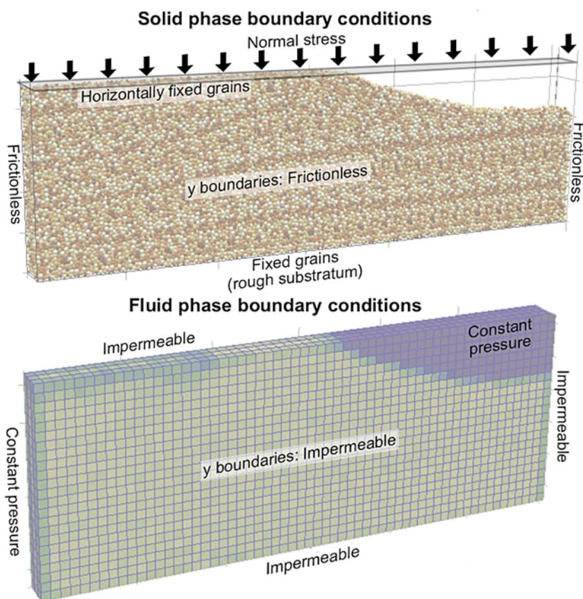
**Fig. 4.** Boundary conditions and initial state in the presented simulations for the granular and fluid phases in the wet experiments.
