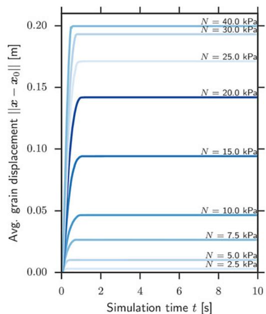
**Fig. 5.** Averaged grain displacements through time for a range of effective normal stresses,  $N$  in the dry granular experiments.
