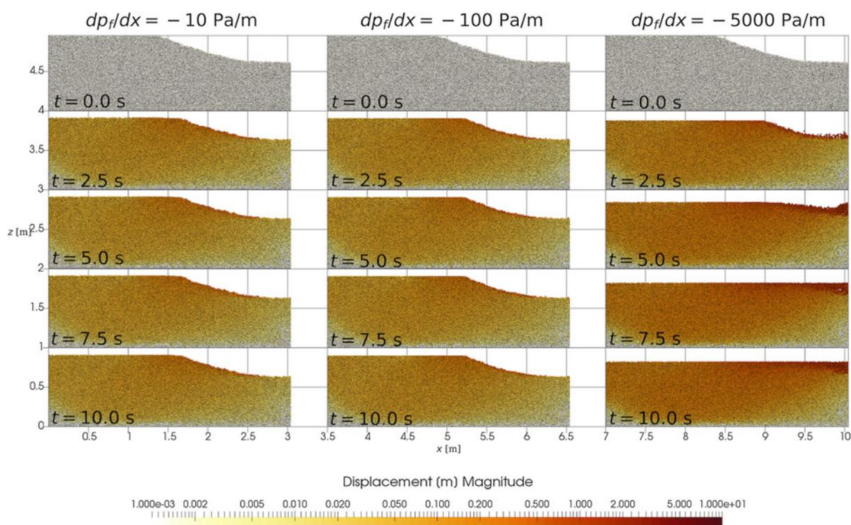
**Fig. 11.** Total per-grain spatial displacements at different times for three wet (water-saturated) simulations with different imposed water-pressure gradients and an effective stress of  $N = 10$  kPa. The water-pressure gradients cause flow and drag forces toward the channel, and destabilize the conduit at higher values.
