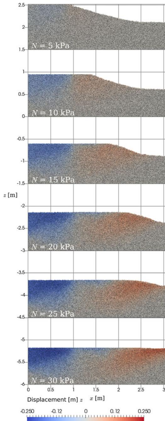
**Fig. 6.** Channel geometries in the steady state at different effective normal stresses  $N$  in dry experiments. Grains are colored according to their cumulative vertical displacement and rendered in an orthogonal projection. The absence of water does not influence the steady-state geometry unless the sediment is flushed by strong water-pressure gradients.
