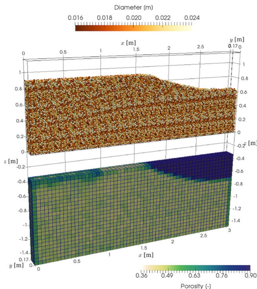
**Fig. 2.** Overview of the granular assemblage of 58 000 particles and the discretization of the fluid grid. We assume symmetry around the channel center (+x) and limit our simulation domain to one of the sides. The model domains of the two phases are superimposed during the simulations.
