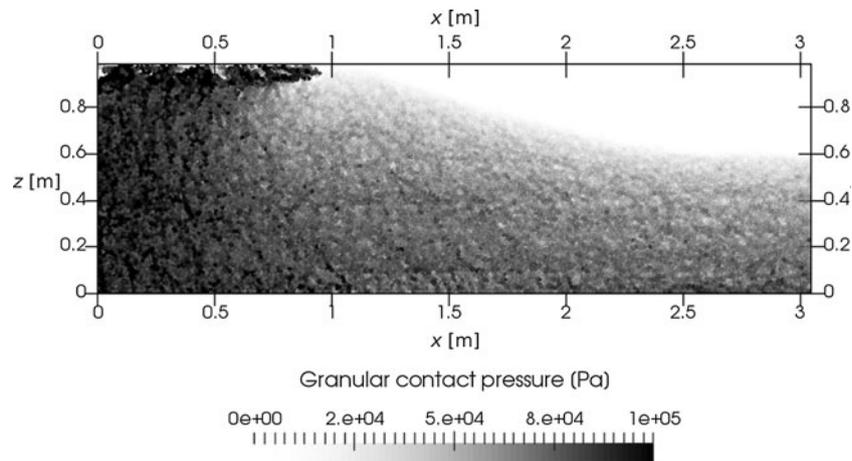
**Fig. 9.** Contact pressure on the grains ( $\sum \|\mathbf{f}_n\|4\pi r^2$ ) in the steady state with an effective stress of  $N = 7$  kPa.
