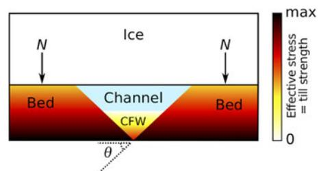
**Fig. 8.** Idealized schematic of effective stress magnitude and till yield strength in a cross-section around a subglacial channel incised in the sedimentary bed. Sediments beneath the channel floor are not stressed by ice weight on the flanks, and comprise a weak channel floor wedge (CFW).
