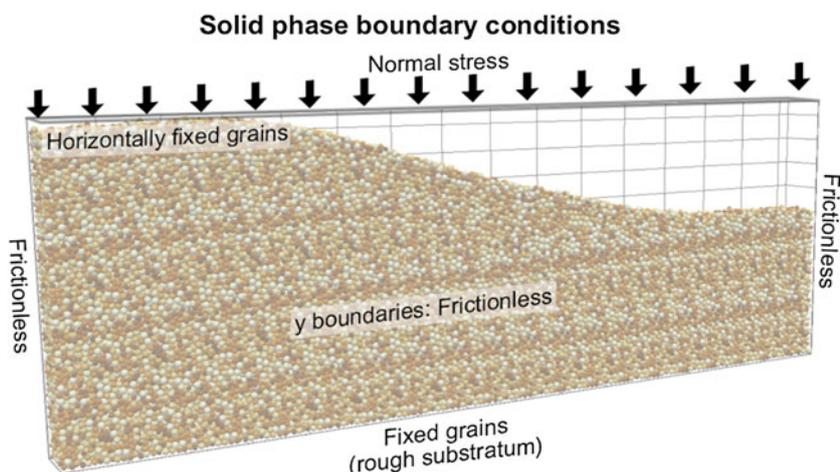
**Fig. 3.** Boundary conditions and initial state in the presented simulations for the granular phase in the dry experiments. The frictionless lateral boundaries imply no boundary-parallel movement.
