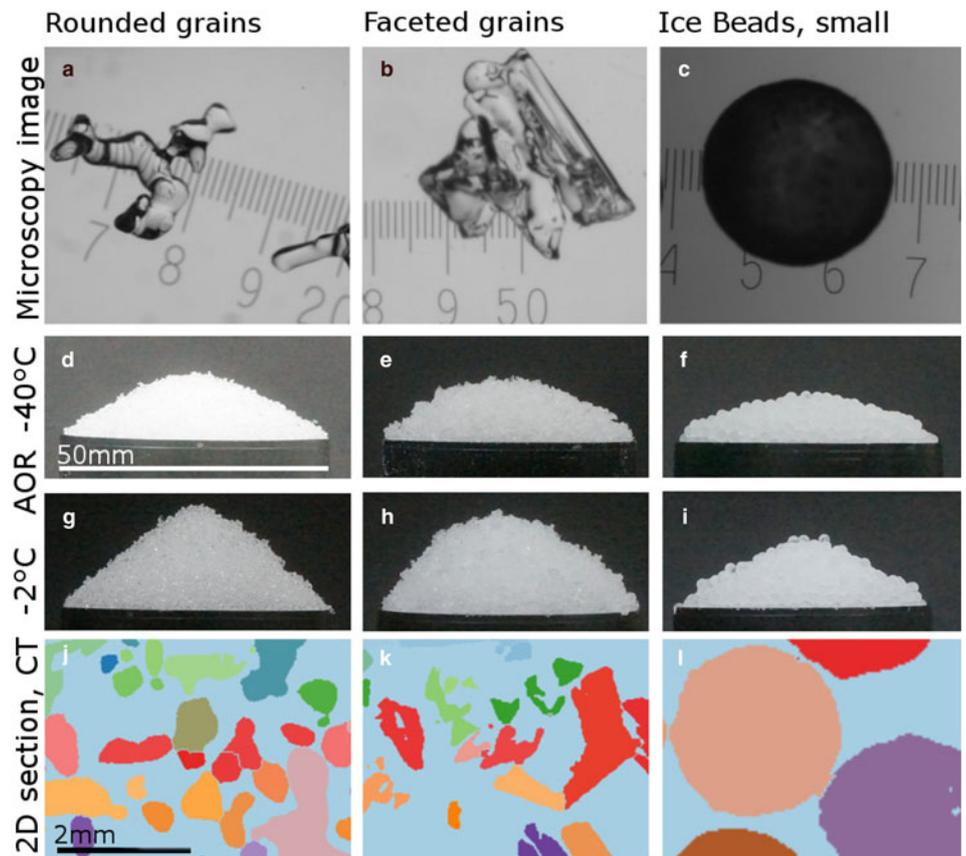
**Fig. 1.** Investigated snow samples in the columns; from left to right: RG, FC, IBS. In the rows: 1 (a)–(c) Microscope image of one representative grain (scale in mm). In row 2 (d)–(f) exemplary heaps showing the angle of repose (AOR) at  $-40^{\circ}\text{C}$  (RG at  $-30^{\circ}\text{C}$ ) and in row 3 (g)–(i) heaps at  $-2^{\circ}\text{C}$ . Row 4 (j)–(l) shows 2D section of 3D  $\mu\text{CT}$  images after binary and watershed segmentation (same scale).
