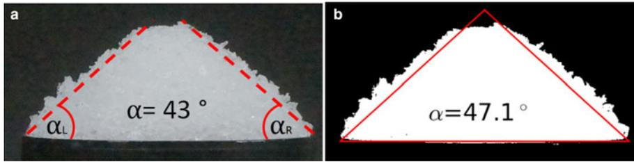
**Fig. 2.** Determination of the angle of repose  $\alpha$  from the images with two independent methods: (a) shows the evaluation of the two lateral slopes with a line drawn by eye (method (a)); (b) shows the projected heap area to calculate the angle of ideal area-equivalent triangle (method (b)).
