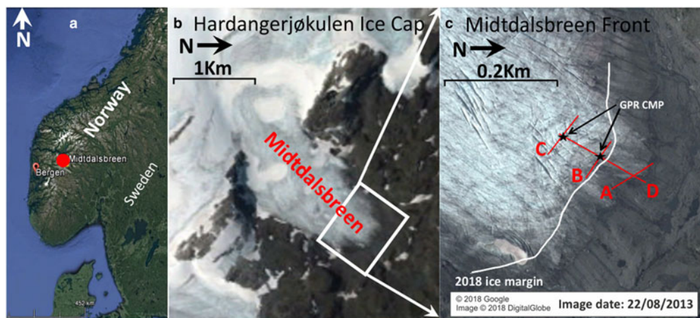
Fig. 2. (a) Location of Hardangerjøkulen ice cap, South Norway. (b) Google Earth image of Midtdalsbreen, an outlet glacier of the Hardangerjøkulen ice cap. (c) Survey lines acquired during the 2018 field season at the front of Midtdalsbreen. Google Earth satellite images taken in 2013. Note that (b) and (c) are orientated away from north to enable optimal data comparison in later figures.
