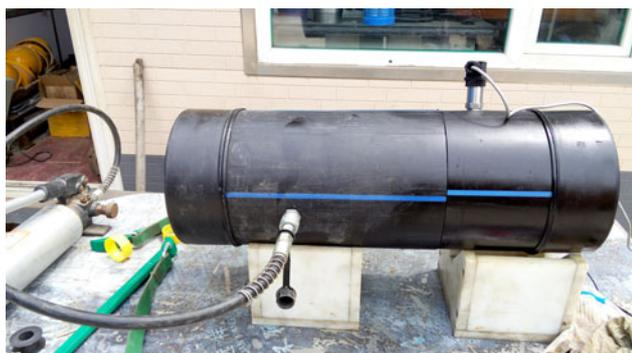
Fig. 16. Pressure testing of casing connections.
