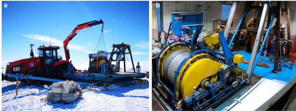
Fig. 5. Drilling winch system: (a) unloading into the movable drilling shelter at Zhongshan Station, Antarctica and (b) view of the drilling winch inside the shelter.
