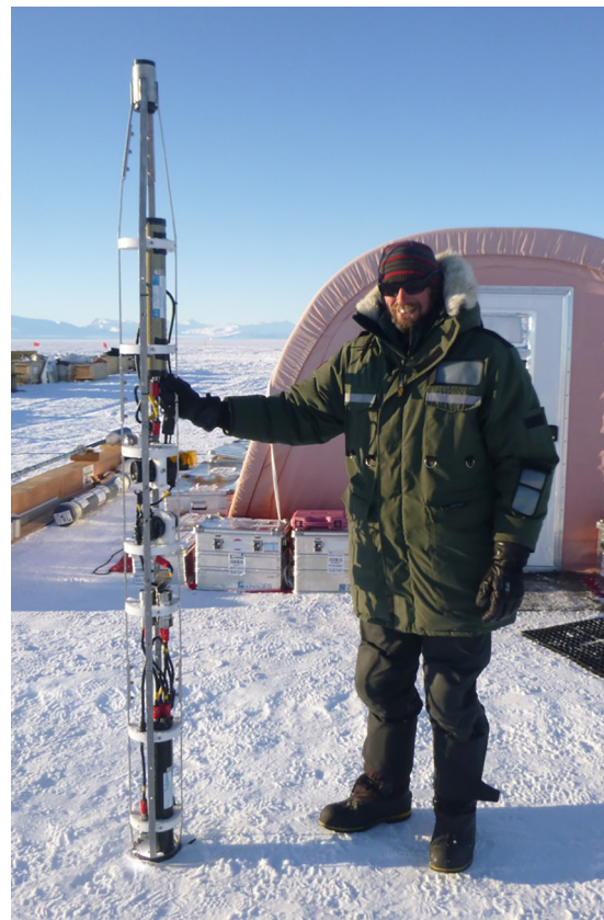
Fig. 18. DHI package prepared for tethered deployment.
