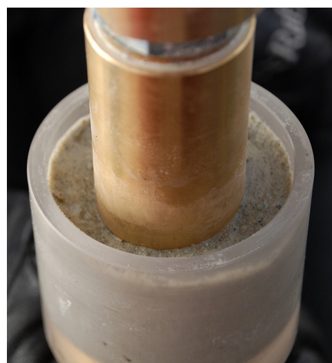
Fig. 22. Nozzle sediment cup with collected sediment, shown immediately after the first return of nozzle to surface at Hole 2.
