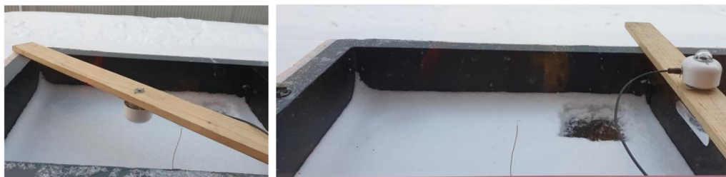
Figure 4. Top view of the second compartment during C2-T01 showing the pyranometer position when recording reflected radiation (left) and the pyranometer position between two compartments when recording the incident radiation (right).
