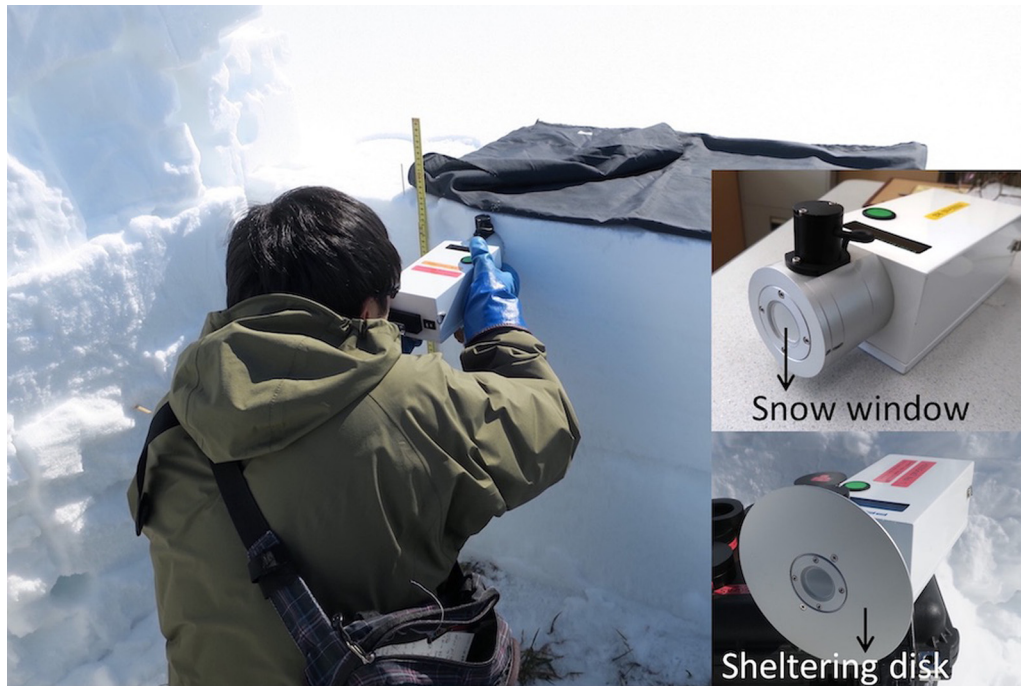
Figure 1. Direct measurement of a snow pit face with the HISSGraS instrument. A black cloth covers the snow surface to protect against stray light from solar radiation entering the HISSGraS instrument. The inset photo at top right shows the front of the HISSGraS and the glass window (snow window) installed in the open port of the IS. The diameter of the window aperture is 25 mm. The inset photo at bottom right shows HISSGraS with a sheltering disk attached to prevent stray light from penetrating through the snow surface during the snow surface measurements. The diameter of the sheltering disk is 150 mm.
