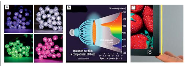
**Figure 3.** Quantum dots (QDs) as optical down-converters. (a) Holiday lights introduced by Evident Technologies in 2008 used blue light-emitting diodes (LEDs) to excite a mixture of CdSe/ZnS QDs dispersed in a polymer matrix. (b) Red-emitting QDs placed in front of a LED improve the quality of white light by increasing the color rendering index and reducing the correlated color temperature. (c) Color IQ optical components can be found in 2013 Sony TV models.<sup>53</sup>
