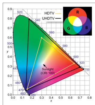
Figure 2. International Commission on Illumination (CIE) chromaticity diagram used to quantify the quality of color for displays, TVs, and other technologies. The yellow triangle represents the HDTV color gamut standard, and the black triangle shows the color gamut for the ultra HDTV standard. In both cases, three primary colors (red, green, and blue) are mixed to obtain the entire color palette. Adapted from Reference 52.
