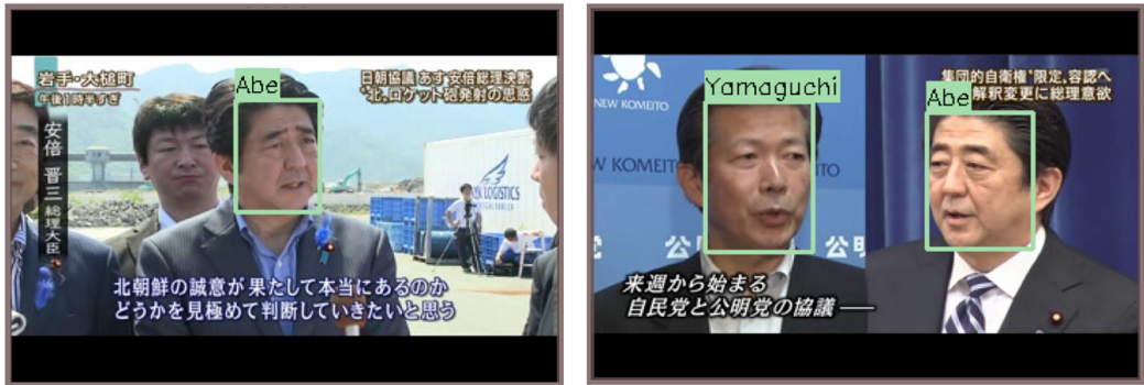
Figure 4. Annotation examples for U.S. TV and Japanese TV annotations. The U.S. TV dataset consists of a single face annotation per frame, whereas in the Japanese TV dataset, all individuals of interest are annotated in every frame. Green bounding boxes indicate the annotated ground truth data.
