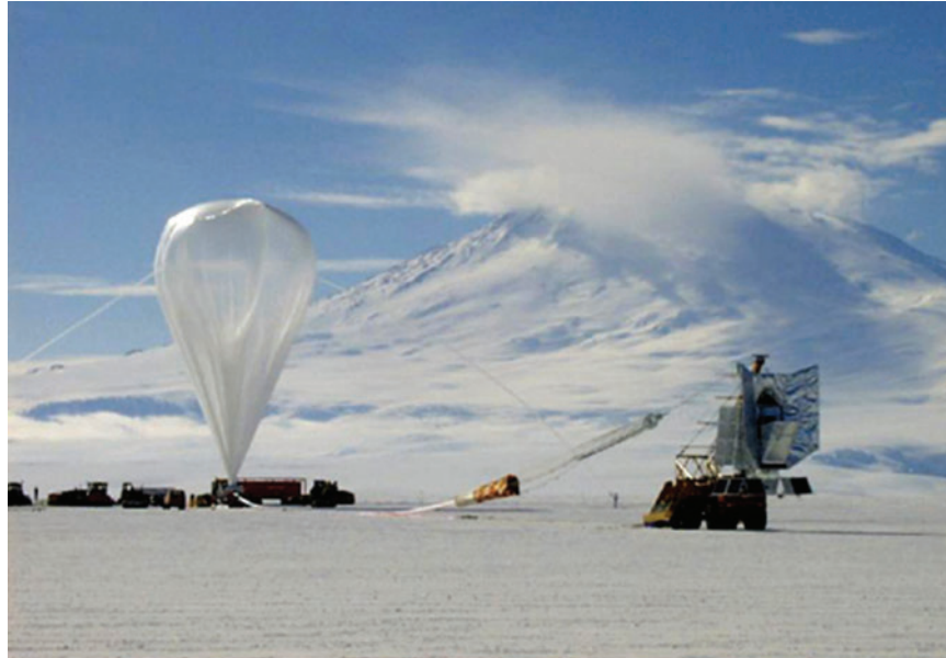
Figure 10 The BOOMERanG experiment, being launched from the US coastal station McMurdo in December 1998. BOOMERanG carried a 1.2-m microwave telescope to an altitude of 38 km by a balloon, and was the work of a US/Italian team. Image provided by Office of Polar Programs, National Science Foundation, 1998.
