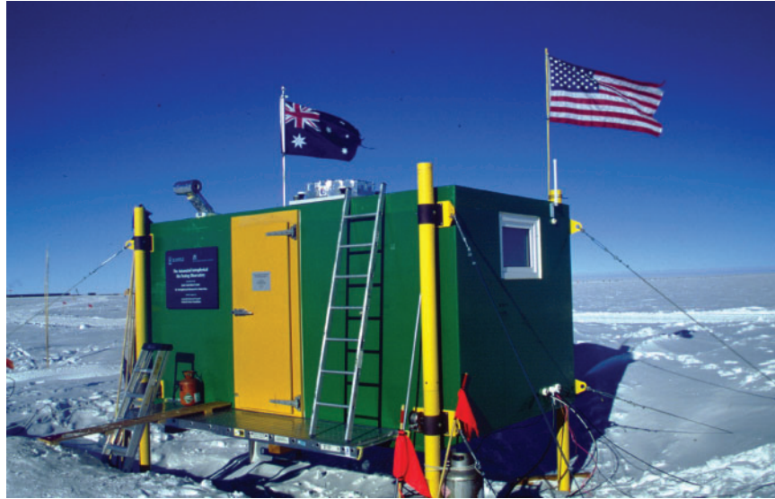
Figure 5 The AASTO, installed at the South Pole in 1997. This self-powered, autonomous laboratory hosted a suite of site-testing instruments for the purpose of quantifying the performance of the site for astronomical use. Picture credit: Michael Burton, 1999 January.
