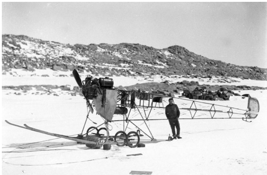
Figure 2 The air tractor used in the 1911–14 Australasian Antarctic Expedition, designed for towing of equipment on sleds, with its engineer Frank Bickerton, discover of the Adelie Land Meteorite. The air tractor only functioned for a few hours, however, on Bickerton's Western Sledging Party, before its pistons seized up. Picture credit: Mitchell Library, State Library of New South Wales, ref. ON 144/H475.
