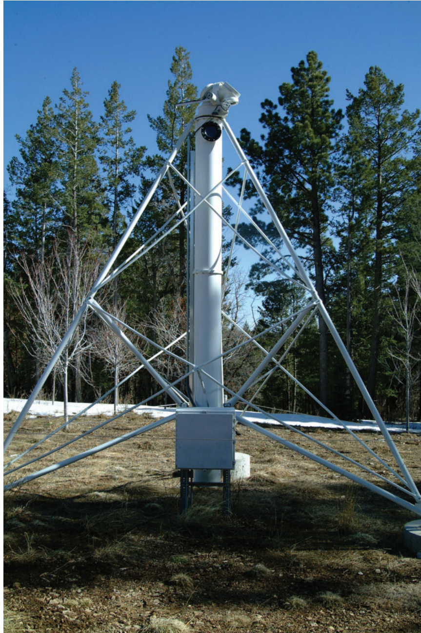
Figure 7 The SPOT telescope, a 2" telescope which was the first optical telescope to be operated through the winter at the South Pole. It is shown as it is currently installed, at the Sunspot Solar Observatory, New Mexico, USA. Picture credit: Balthasar Indermuehle, 2002 November.
