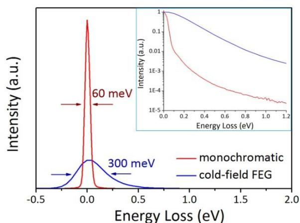
Figure 1. Comparison of the ZLP taken on the Nion UltraSTEM with and without the monochromator. The main figure is normalized to the integrated intensity, while the inset is normalized to the maximum intensity of the ZLP.
