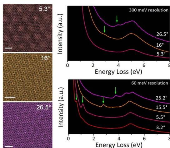
Figure 2. (Left) Experimental ADF images of twisted bilayer graphene with different misorientation angles. Scale bars: 1 nm. (Right) Low-loss EEL spectra of the TBG acquired using the Nion UltraSTEM with and without the monochromator. The misorientation angles are labeled on each spectrum.
