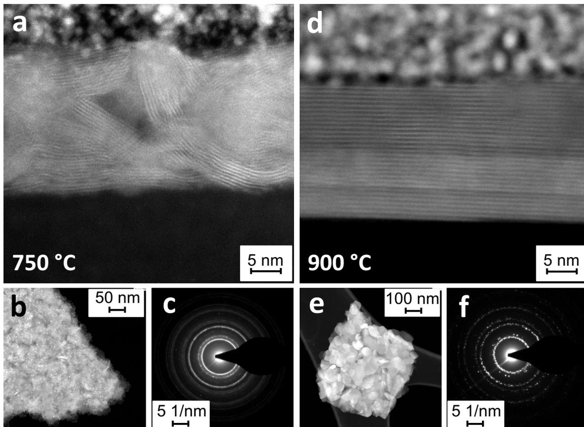
**Figure 1.** TEM analyses of fabricated MoS<sub>2</sub> films annealed at 750 °C: (a) the cross-section STEM image, (b) planar view reveals no distinct grain boundaries and (c) shows its diffraction pattern. MoS<sub>2</sub> films annealed at 900 °C revealed (d) uniformity in the interlayer spacing with (e) distinct grain boundaries and (f) the diffraction pattern taken from the planar view (e).
