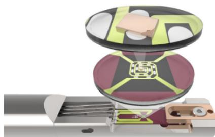
**Figure 2.** Schematic of the heating DENS Wildfire holder used for in-situ heating.
