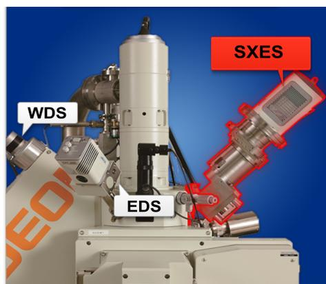
**Figure 3.** The JEOL EPMA JXA-8320 with attached WDS, EDS and SXES.
