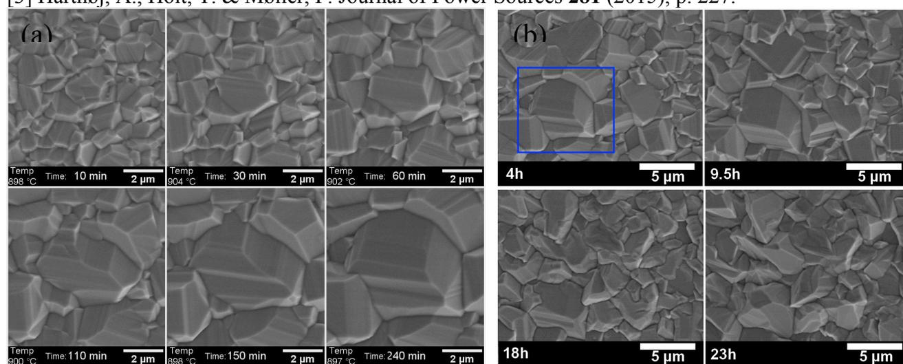
**Figure 1.** (a) grain growth at the surface of the sample at 900°C under 30Pa of O<sub>2</sub>. (b) Morphology change after 4-23h exposure to same condition (blue rectangle highlight the grain that growth is showed on (a)).
