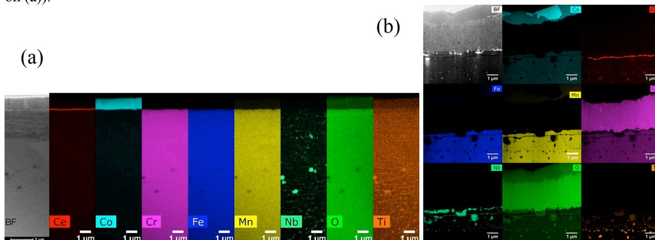
**Figure 2.** STEM EDX of the cross section of the surface of the coated steel (a) before oxidation and (b) after 48 hours oxidation at 900°C under 30Pa O<sub>2</sub>.
