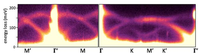
**Figure 2.** ω-q experimental diagram obtained from hexagonal BN in two parallel acquisitions (left) spanning  $\Gamma$ -M- $\Gamma$ '-M' and (right)  $\Gamma$ -K-M'-K'- $\Gamma$ '. The curves show clearly the dispersion of the phonon energies as a function of momentum. 30 kV, 15pA, 20 meV resolution,  $\alpha/2=1.5$  mrad, collection full-angles  $\beta_1$  x  $\beta_2$  approximately 3 mrad x 50 mrad.
