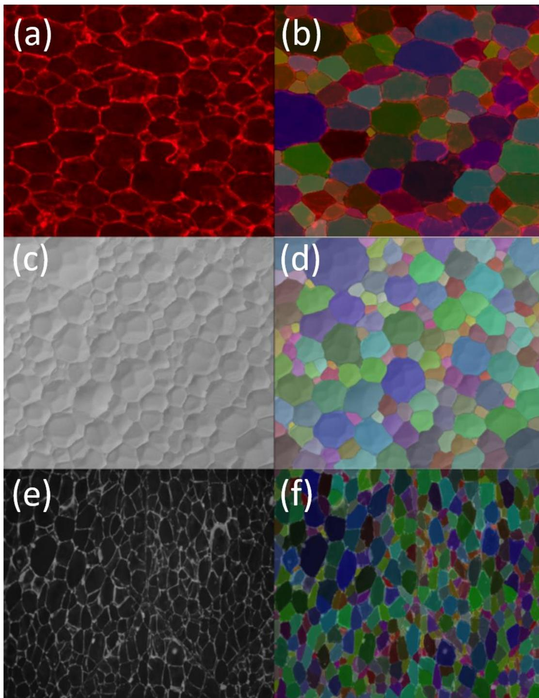
**Figure 1.** (a) An optical image of a polyisocyanurate foam, (b) image (a) with the identified cells color-coded, (c) a scanning electron microscopy image (back-scattered electron image) of a poly-isocyanate foam, (d) image (c) with the identified cells color-coded, (e) an optical image of an expanded polystyrene foam sample after transformed from color to gray scale, (f) image (e) with the identified cells color-coded.
