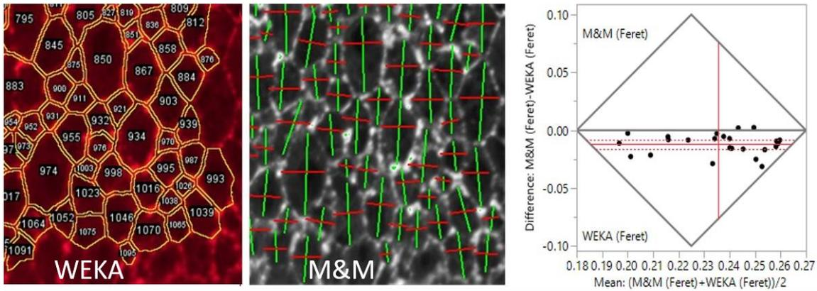
**Figure 2.** Matched pairs analysis of automatic cell size analysis with WEKA (“WEKA”) and manual Measure and Mark method (“M&M”) results.
