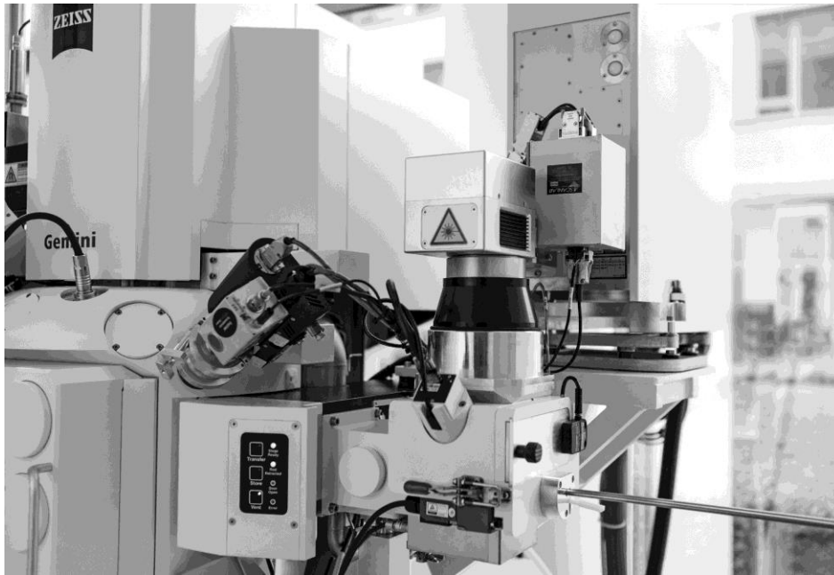
Figure 1. Picture of ZEISS Crossbeam 350 laser with fs laser attached to the airlock.
