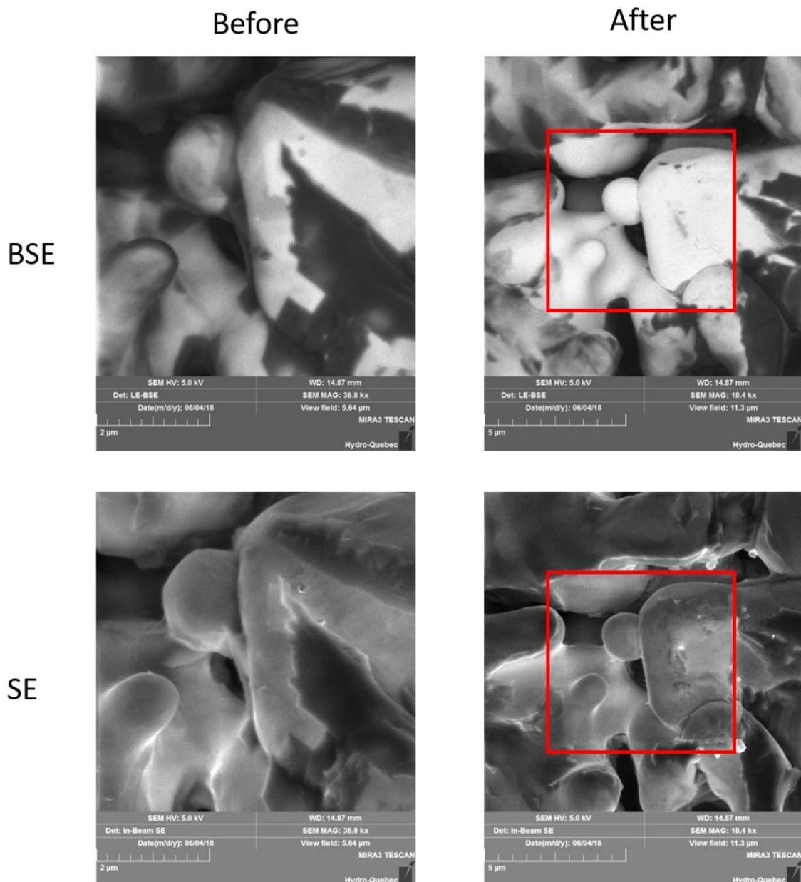
**Figure 1.** Effect of 1 hour acquisition on the LLZO-Ga sample. The red square shows the acquisition area. The BSE micrographs were obtained with low voltage BSE detector and show a compositional contrast of the sample. The SE micrographs were obtained within column SE detector which gives higher resolution topographic contrast, but it is more sensitive to sample charging.
