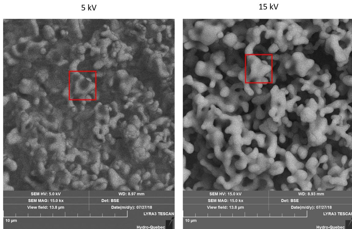
**Figure 2.** The effect of accelerating voltage is shown by comparing two micrographs of the same LLZO-Ga area at 5 kV and 15 kV. The micrographs were obtained with the low voltage BSE detector and show a compositional contrast of the sample. The red square shows a dark phase that is visible at 5 kV, but not at 15 kV.
