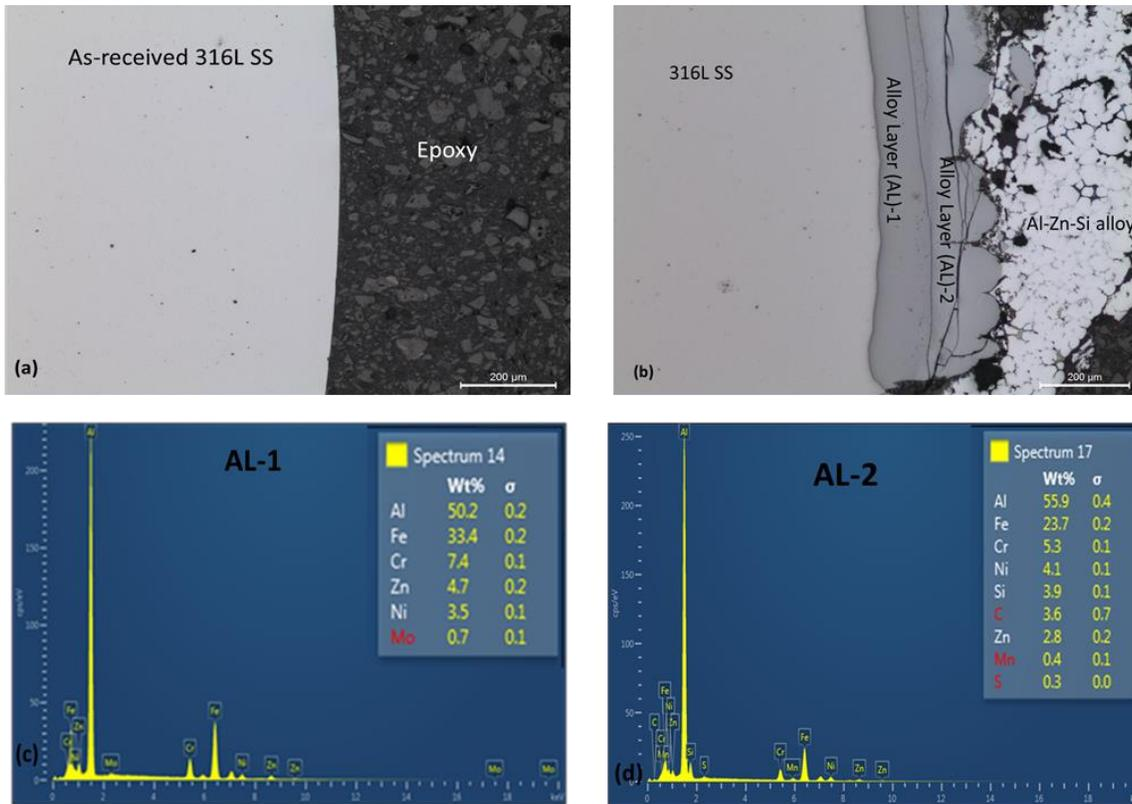
**Figure 1.** Optical microscopic images (a). As-received 316L Stainless Steel, (b). After 7-day hot-dipping, (c). EDS analysis of AL-1, (d), EDS analysis of AL-2
