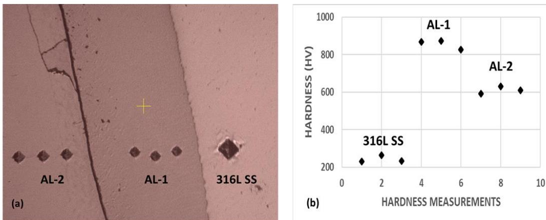
**Figure 2.** Vicker's hardness (HV) testing of 316L Stainless Steel rod hot-dipped for 7 days (a). Optical microscopy image showing indentation marks, (b). HV profile of 316L stainless steel, AL-1 and AL-2
