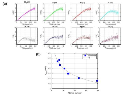
**Figure 2.** (a) Measured relationships of  $\ln(I/I_0)$  vs.t for SiO<sub>2</sub>, Al, Si, Ti, Ni, Cu, Ag with  $\beta$ =16 mrad, t was extracted at multiple locations as indicated in Fig 1b. (b) Maximum thickness  $t_{\text{max}}$  yielding a linear dependence of  $\ln(I/I_0)$  on t from several element with  $\beta$ =16 mrad at 300 keV. Reference
