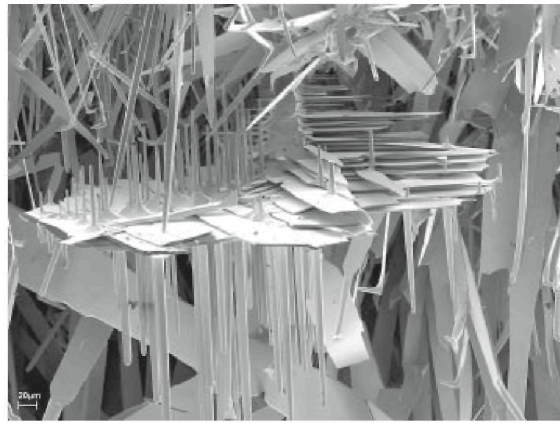
Fig. 5b: Using the HC/DoF module gives a dramatic improvement of the depth of field under the same conditions as in Fig. 5a. Even with a height of 4mm the complete sample is in focus.
