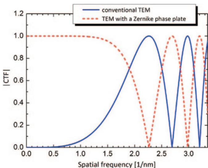
**Figure 2:** Moduli of phase contrast transfer functions (CTFs) without (solid line) and with (dashed line) a Zernike phase plate.  $k_{co}$  is the cut-on frequency of the phase plate determined by the finite size of the central hole of the Zernike phase plate. Parameters for the CTF calculation: defocus 0, spherical aberration 5 nm, accelerating voltage 300 kV.
