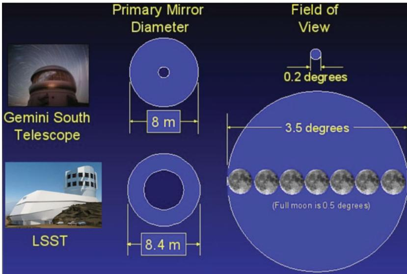
**Figure 1.** A comparison of the primary mirror size and the field-of-view for LSST and Gemini South telescopes. The product of the primary mirror size and the field-of-view, the so-called *étendue* (or *grasp*), a characteristic that determines the speed at which a system can survey a given sky area to a given flux limit, is much larger for LSST. Figure courtesy of Chuck Claver.
