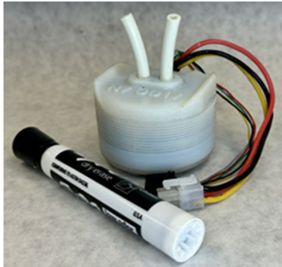
Figure 5. Bidirectional gerotor pump (Gallentine and Barth, 2023). The pump is shown with a dry erase marker for size scale.
