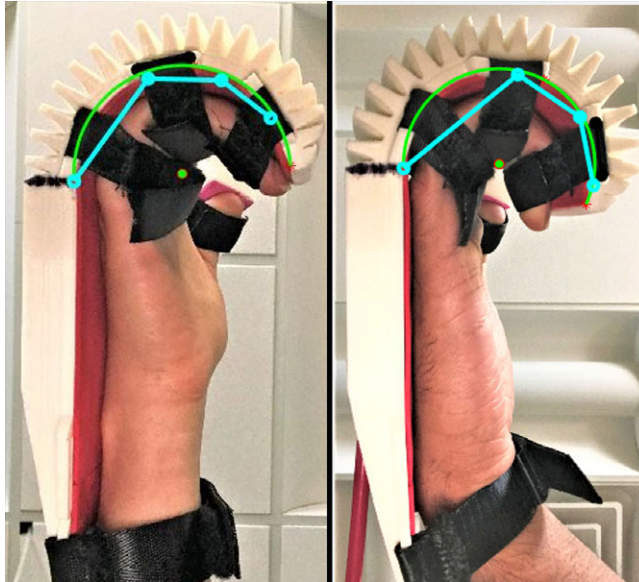
Figure 13. Loaded soft actuator under pressure. This image shows a side view of the orthosis pressurized to 20 psig (left) while worn by the small subject and 32.5 psig (right) while worn by the large subject. Overlaid on the photograph are the actuator curvatures in green, with the center of curvatures as green dots, and the predicted finger profiles in cyan.
