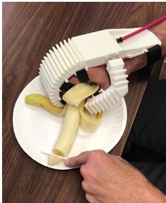
Figure 7. Example ADL: slicing banana. This photograph shows the subject stabilizing and slicing a banana with the help of the orthosis.
