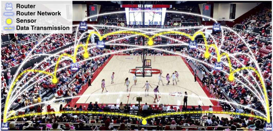
Figure 9. Sensor network design and multi-hop data transmission through routers via WiFi connections at the Stanford Maples Pavilion.
