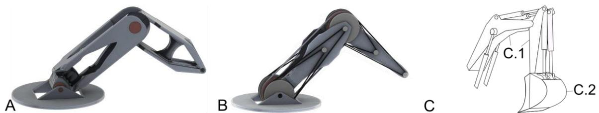
Figure 2. Transfer of tension chording to a simplified robot system (A and B): Reference system (A) and biomimetic tension chording system (B). Boom (C.1) and drag (C.2) of an excavator (C)
