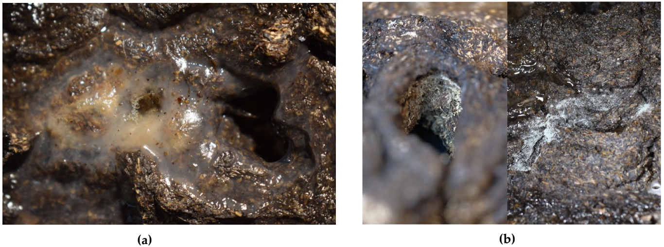
Figure 6. (a) BC growth on sample 5 after 42 days, (b) Examples of contamination occurring on samples no. 4 and 7 (Image credits: authors).
