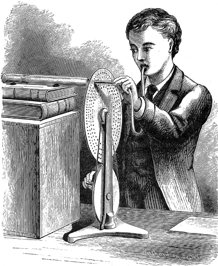
Figure 1.2 A make-it-yourself acoustic siren, much like August Seebeck's, as shown by Alfred M. Mayer (1878). The spinning disk, driven from a crank via string and pulleys, interrupts a stream of air from the tube to make waves of sound pressure that we hear as a tone. Different tones can be made by moving the tube to a different row of holes, or by changing the disk to one with a different pattern of holes. August Seebeck and Hermann von Helmholtz were among the nineteenth-century scientists who used such devices in their research that contributed to connecting the physical and perceptual properties of musical tones to the mechanisms of human hearing—though their theories were somewhat in opposition to each other.
